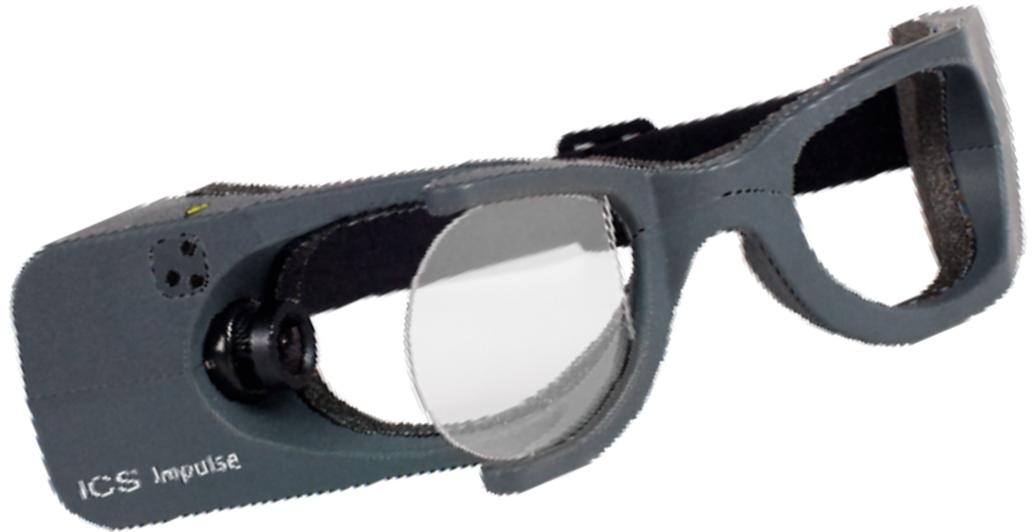
ICS Impulse provides objective evidence of the capacity of each semicircular canal to respond to physiologic velocity stimulus as measured by VOR and saccades.
