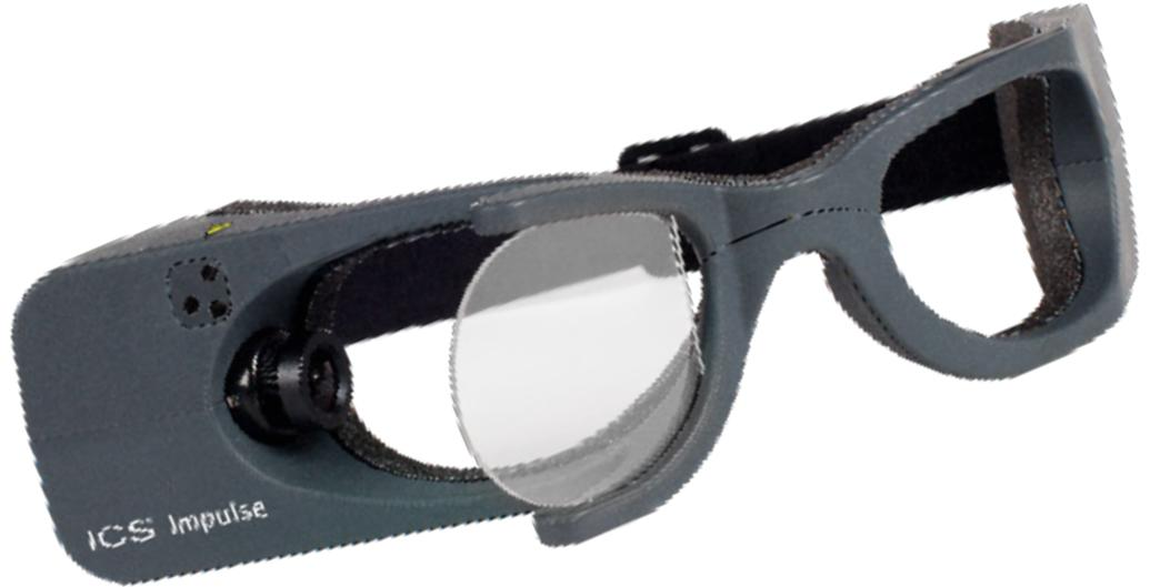
ICS Impulse is an important addition to our vestibular test battery. We use this technology weekly in conjunction with VNG, and VEMP testing, and have seen patient cases where ICS Impulse has made a significant difference. We've had normal VNG results and abnormal Impulse results which ultimately sends the patient on to the best course of treatment.
